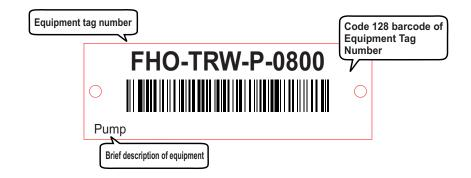
Primark bar code asset tags can be made on both aluminum and stainless steel material. Bar code tags use code 128 symbology (unless otherwise specified).
